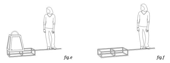
We will need to prevent the frame from tipping and this can be done in a number of ways; by either counterbalancing the frame (*fig.e*) or bolting the frame to the floor (*fig.f*) this being the most acceptable from the designers point of view and leads us to our next problem:
