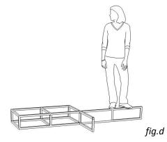
So we have now arrived at *fig.d* a design a long way from the original, but one that will prevent the frame from tipping and be able to support the load.
